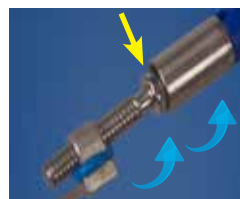
Fig 15. To lock into place turn the safety screwdriver clockwise.
